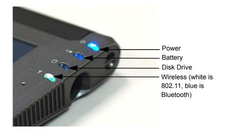
The front panel LEDs are described in the following table.
